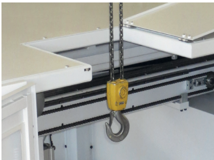
Top loading door for crane operation.
